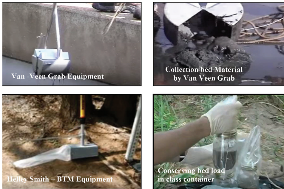
Figure 5. Sampling bed load material
