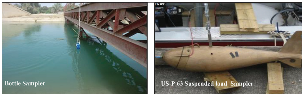
Figure 4. Sampling devices to measure suspended load
